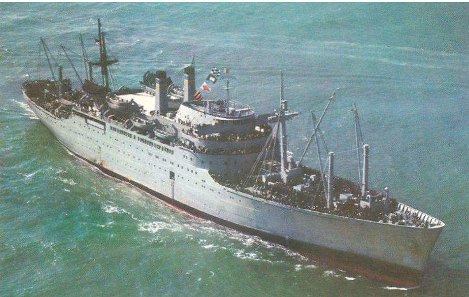
↑ This aerial view of the USNS Barrett shows the ship's distinctive superstructure to good advantage. Note that the blue and gold bands were painted on the uptakes rather than on the dummy funnel as was customary.
